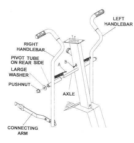
**7.** With PIVOT TUBES on rear side of HANDLEBARS and CONNECTING ARMS to inside, slide RIGHT and LEFT HANDLEBARS onto AXLE. Slide LARGE WASHER onto end of AXLE. Carefully tap PUSHNUT onto end of AXLE with hammer. Connect heart rate wires from CONSOLE TUBE (B) to heart rate wire in each handlebar (A).
